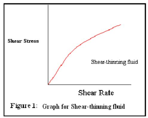
We describe the relationship between the shear stress  $\tau$  and shear rate  $\theta$  as follows:
